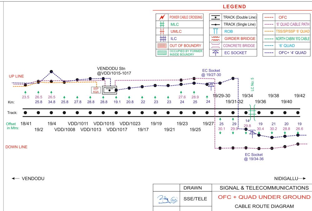
NOTE: - MEASUREMENT IN METERS FROM CENTER LINE OF THE TRACK.
