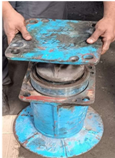
Housing of spring pads, check sleeve, buffer washer, shims inside plunger
