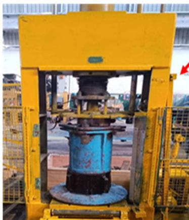
Compressing the buffer pads and base plate in hydraulic press
