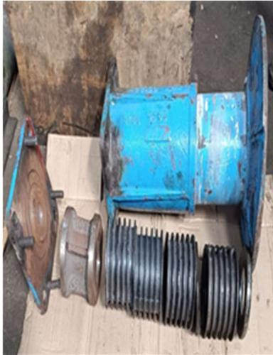
Dismantled Buffer assembly components
