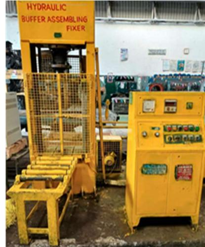
Hydraulic Buffer assembling fixture
