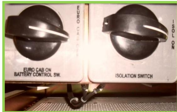
Battery control switch (OFF position) ✦ TPWS isolation switch (ON position)
