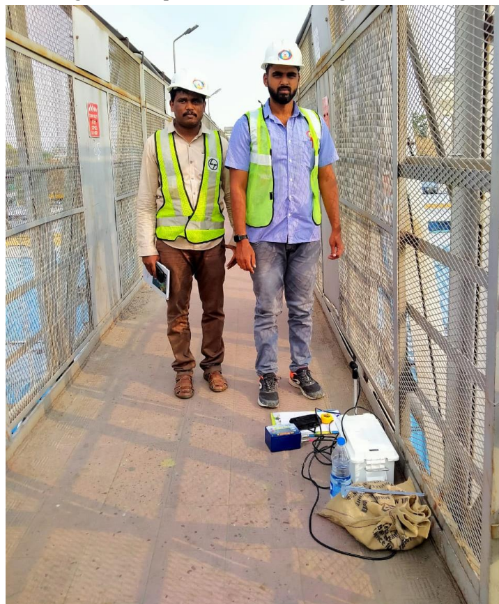
Fig 1.11: Vibration Test at Kachiguda FOB
