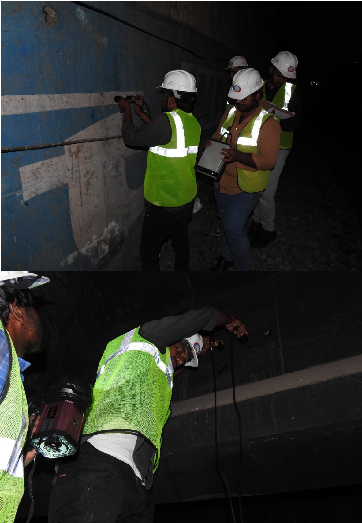
Fig.6.1 UPV test at site
