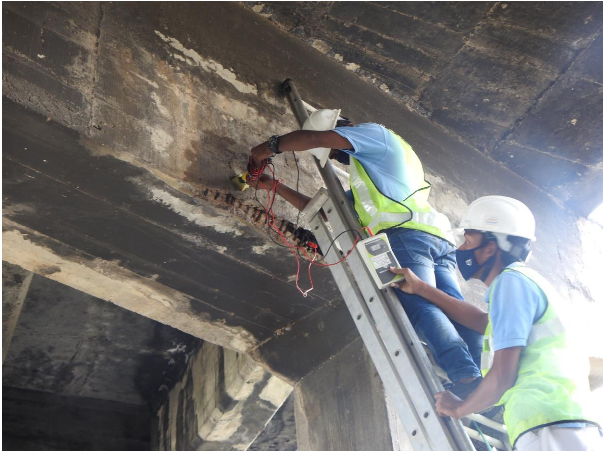
Fig 17: Half-cell potential test at site
