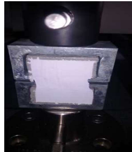
Crack Bridging Test on Dekguard E2000
