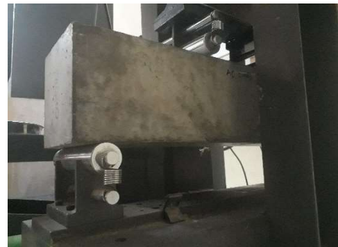
Beam reinforced with 2 Laminates on soffit
