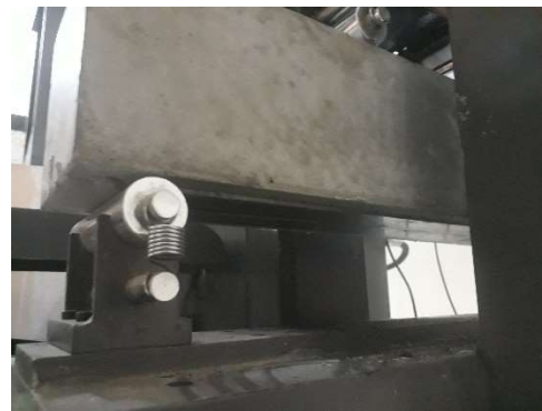
Beam reinforced with 2 Laminates on soffit
