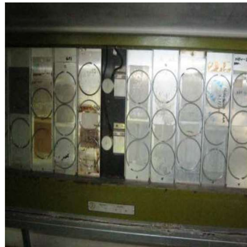
QUV – 8hrs UV, 4hr condensation
