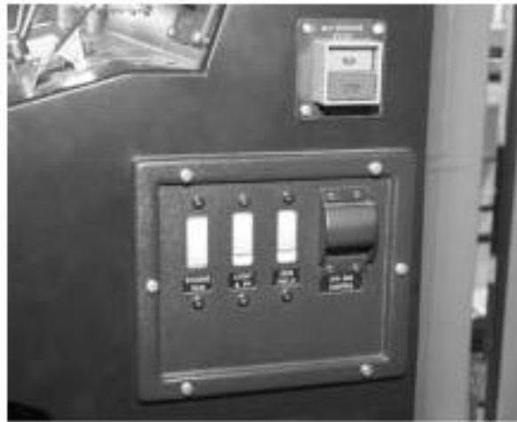
Figure 2-14. MU ENGINE STOP Switch (top), and Control & Operating Switch Panel with DYN BRAKE CONT CB
