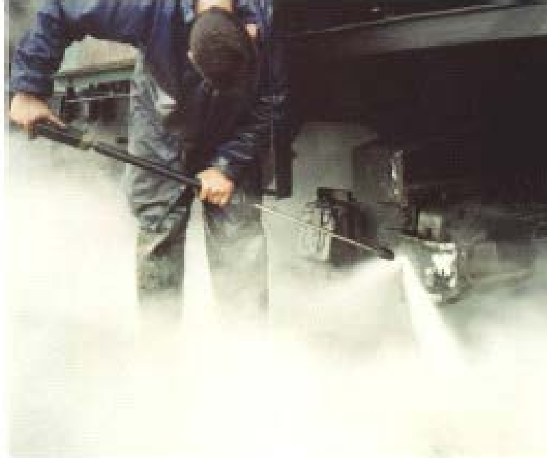
Figure 5.2.2.1: Example of pre-cleaning a part with high-pressure steam.
