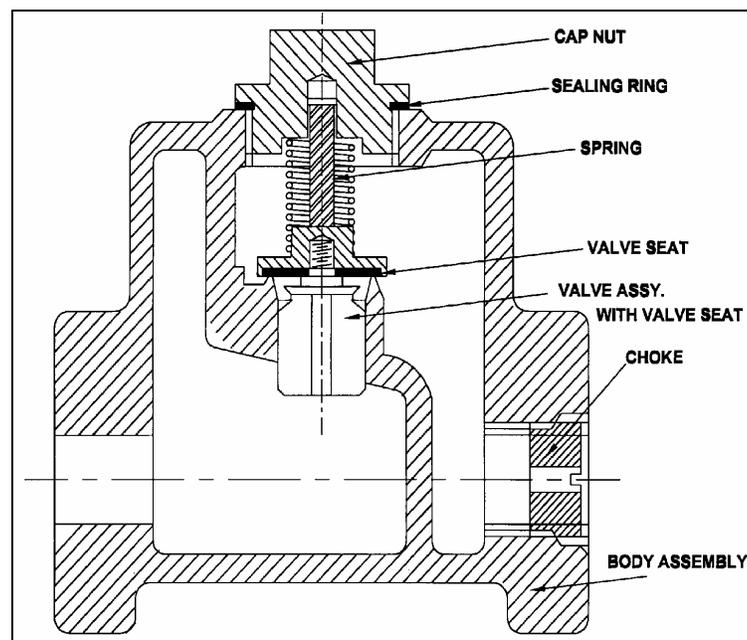
Figure 4.21 CHECK VALVE WITH CHOKE
