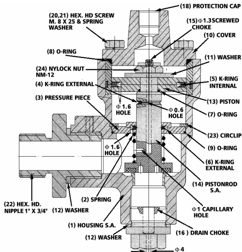
**Figure 4.20 : PASSENGER EMERGENCY ALARM VALVE ASSEMBLY**
