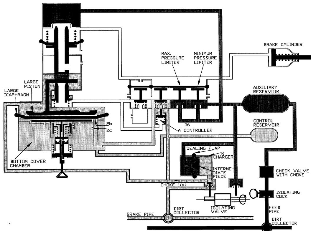
**Figure 4.16 - KE DISTRIBUTOR VALVE (CHARGING STAGE)**
