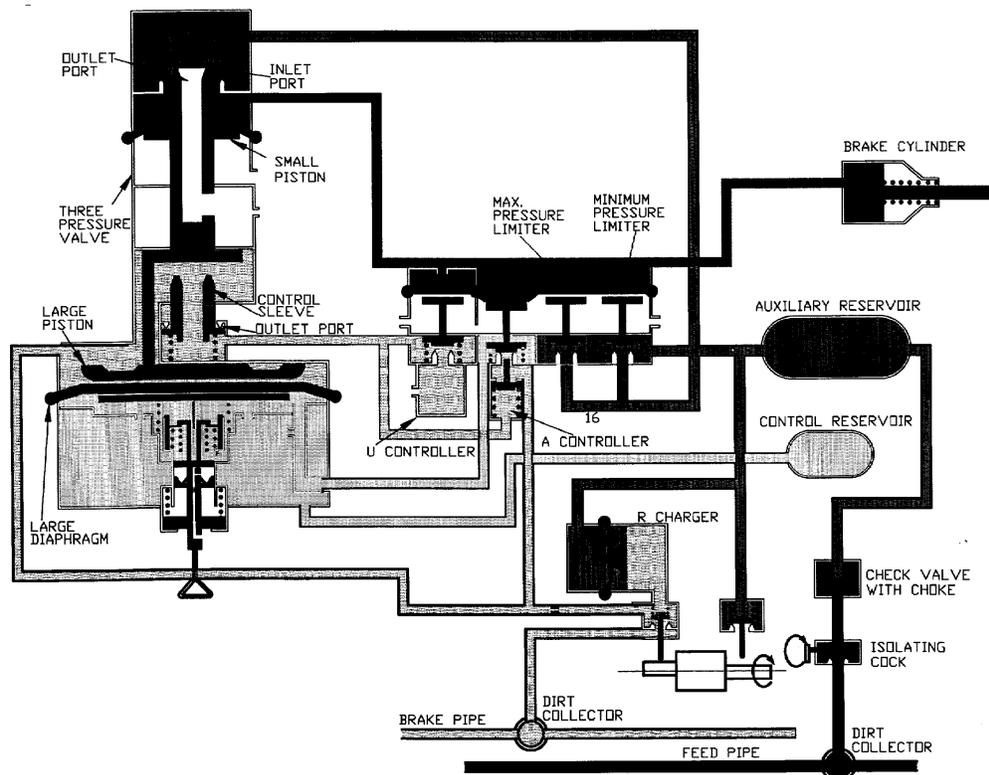
**Figure 4.17 - KR DISTRIBUTOR VALVE (GRADUATED APPLICATION)**
