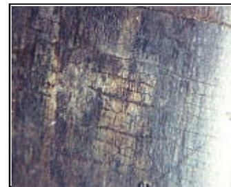
during normal braking. Such wheels do not need to be withdrawn but should be carefully distinguished from the rejectable thermal cracks.
