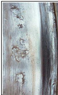
These are generally associated with small skid marks or “chain sliding.” Such wheels should be withdrawn from service and sent to workshops for reprofiling.
