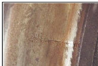
service. If a crack becomes visible on the outer flange face, the wheel should be withdrawn from service. Such wheels should be sent to workshop for examination and subsequent rejection.
