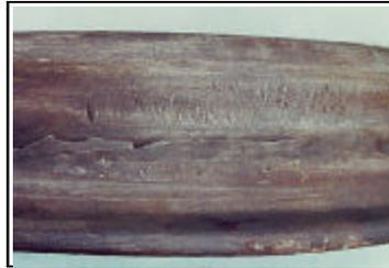
**3. Shelled Tread** - Shelling can be identified by pieces of metal breaking out of the tread surface in several places more or less continuously around the rim. Shelling takes place when small pieces of metal break out between the fine thermal checks.
