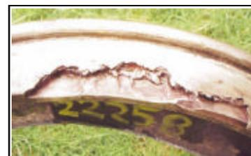
2. **Spread Rim**- If the rim widens out for a short distance on the front face, an internal defect may be present. Spreading of the rim is usually accompanied by a flattening of the tread, which may or may not have cracks or shelling on the tread. Such wheels must be withdrawn from service.
