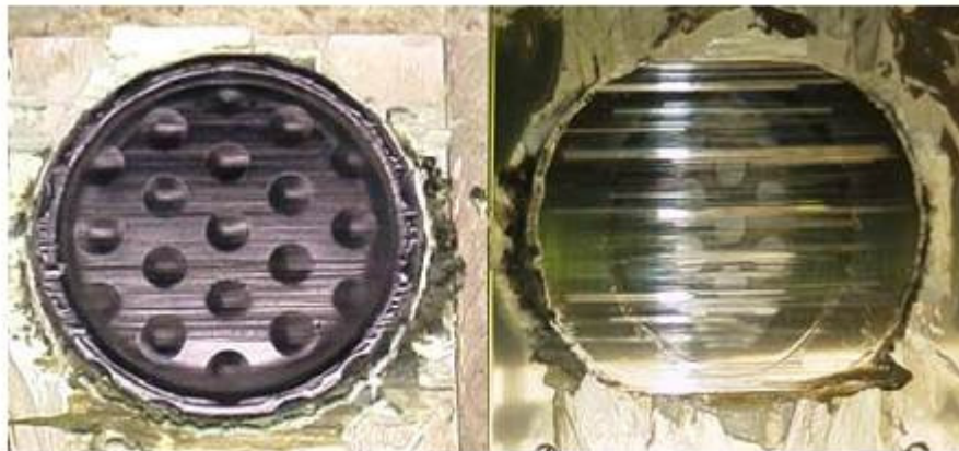
Condition of UHMWPE sliding surface after testing in laboratory
