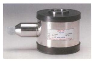
various ranges from 100 to 5000 KN. The change in pressure on the diaphragm will change the tension of vibrating wire. The natural frequency of wire is proportional to the tension of the wire. Thus, by measuring the natural frequency of wire pressure on diaphragm can be known. Natural frequency of the wire can be co-related with the diaphragm pressure. The natural frequency of wire can be expressed as below:
