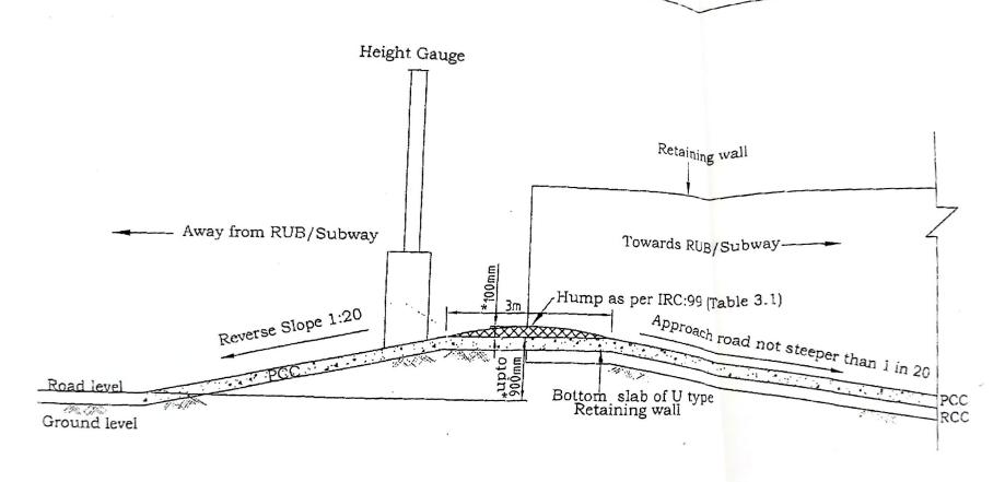
Schematic Arrangement for Reverse slope with Hump
